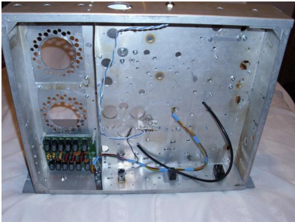
Start of underside wiring. The tuned input board, bias board, and the start of the air ducting.
