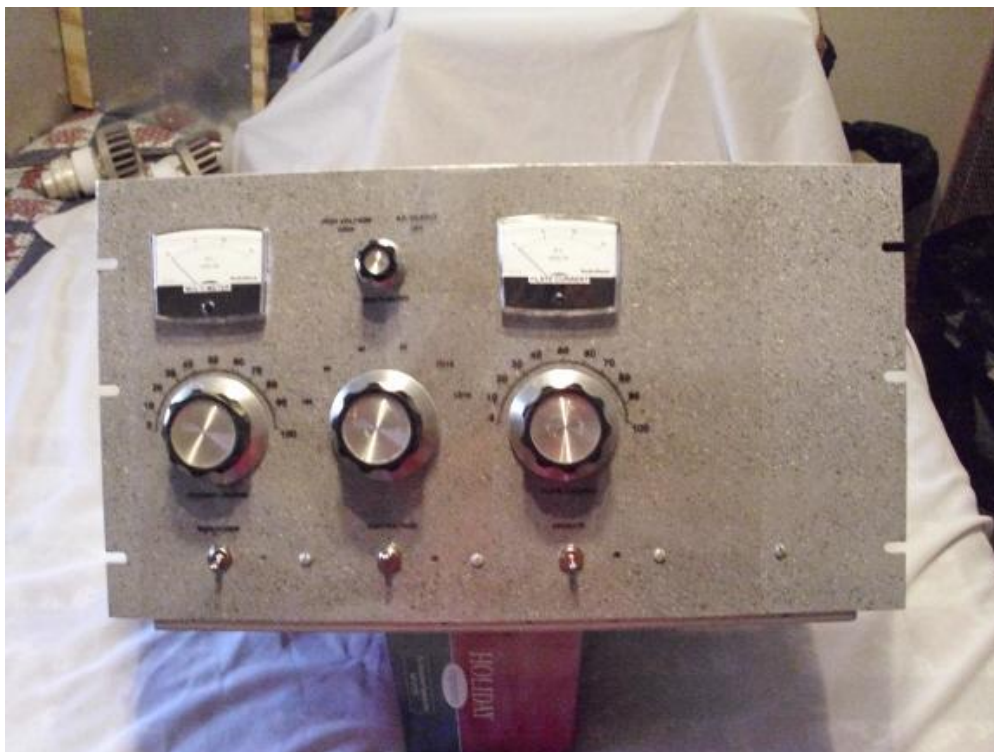
As of 28 June 2011: The amplifier has a long way to go. However, the front panel is now lettered using overhead transparencies printed on an inkjet printer.
