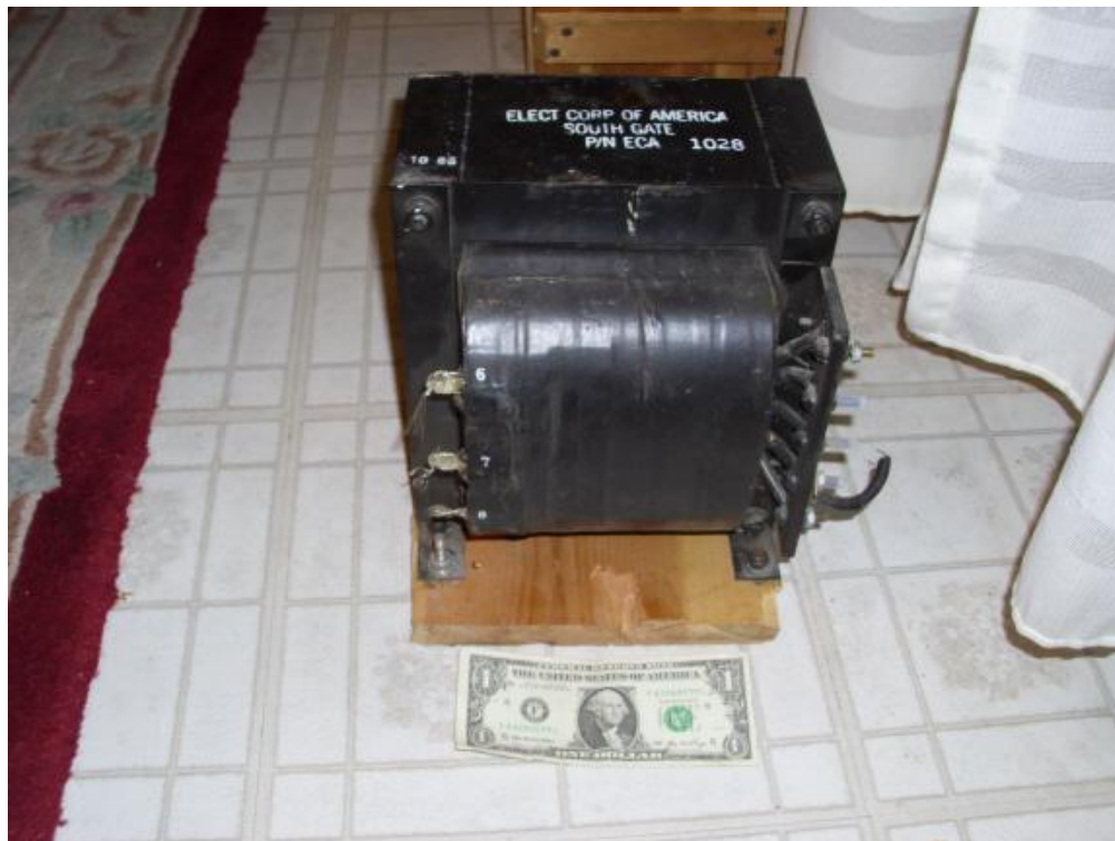
High voltage transformer
