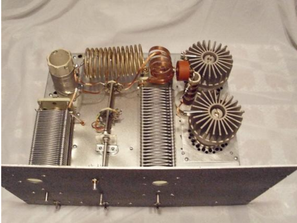
Revised pi-network layout. The 160-meter and the 15, 12, 10 meter coils were moved to shorten the connections to the bandswitch. Also, the wires between the coils and the bandswitch were replaced with copper braid.
