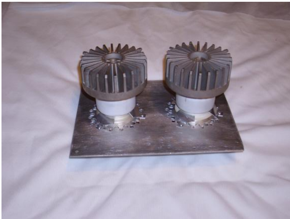
Diagram of hold down clamp (holds tube to socket plate)
