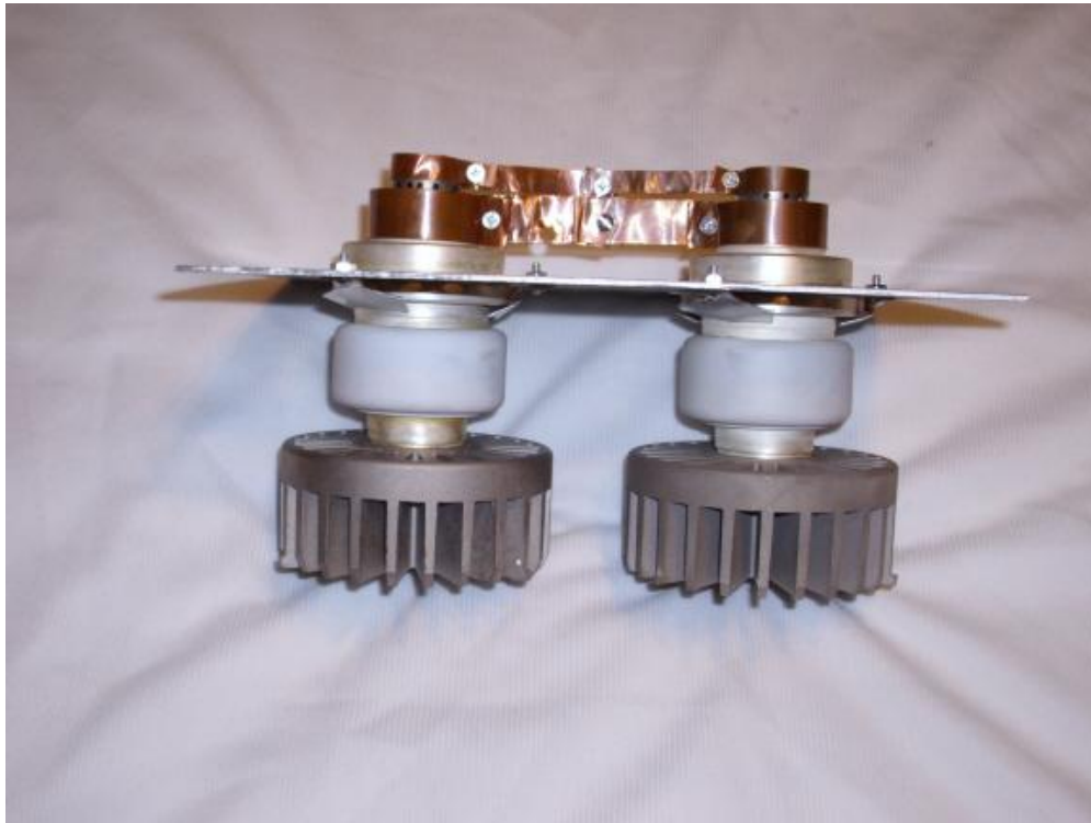
View showing cathode and heater connections
